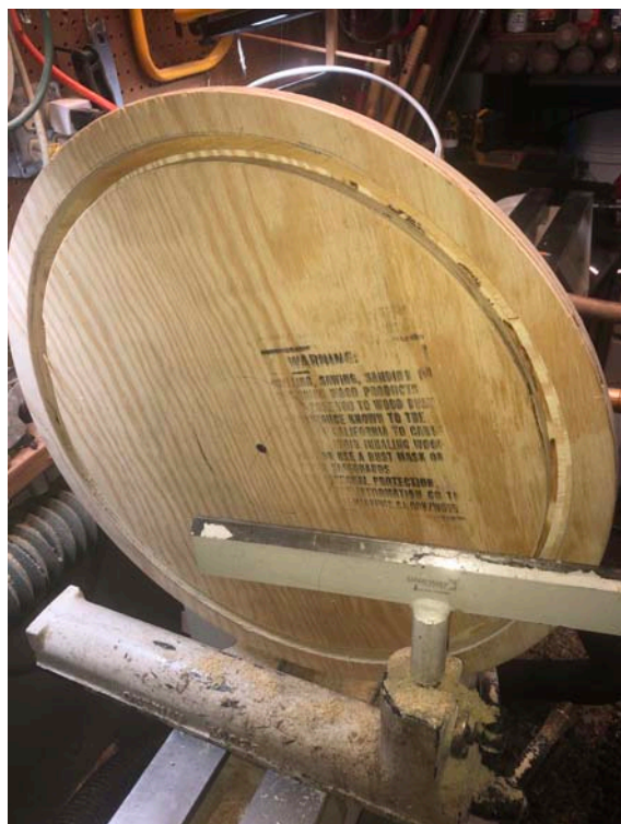
Adapter ring: 3/4" plywood 20-3/16"od.
