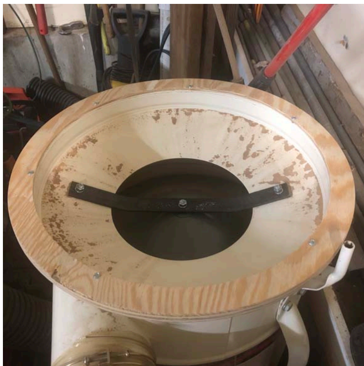
Adapter ring in place with. Conical vortex mounted in the inlet section.
