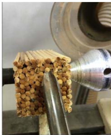
4 Against the grain. As the blank continues turning, the gouge now cuts endgrain, lifting or tearing the unsupported fibers; the surface is rough.
