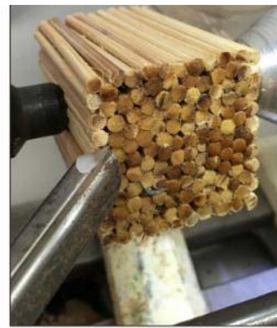
5 Across the grain. Cutting across the grain from left to right, the fibers are supported by those next to them; the cut surface is smooth.
