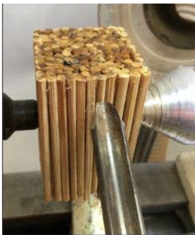
4 With the grain. As the blank comes around from sidegrain to endgrain, the gouge will cut the supported fibers, leaving a clean surface.
