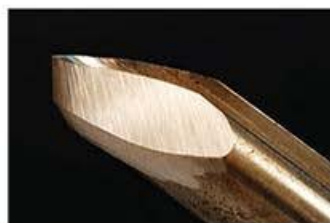
This \frac{3}{8} " bowl gouge has a fingernail grind.
