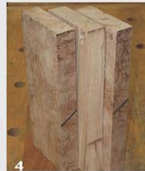
4 Position the waste wood between the halves of the resawn goblet blank.
