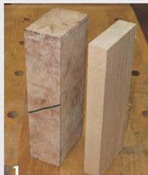
1 Mark the goblet blank with an angled line for easy reference at glue-up time.
