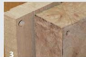
3 Drill matching alignment holes in the waste wood.
