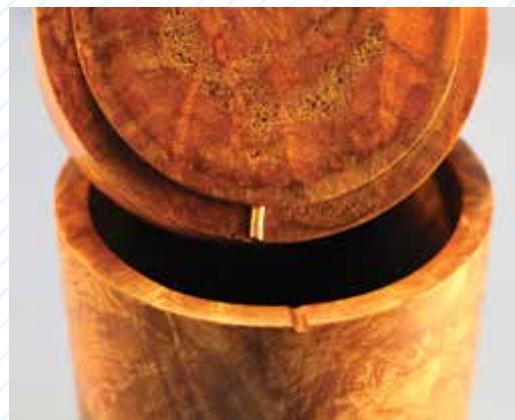
An unobtrusive pin affixed at the box/lid juncture registers the lid at the correct grain orientation.
