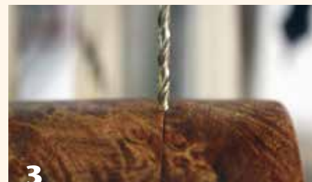
Tape the lid to the box securely before drilling. Use a shopmade V-block to hold the round box and then drill a pinhole centered on the box/lid juncture.
