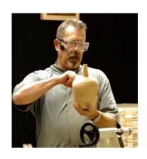
Flip the piece around on the lathe so that the bottom of the piece is chucked at the head stock. Then start working ons the shape of the piece, make it a genie bottle or any shape you want but one that will tend to support the illusion of having been hollowed through whatever opening you create. Reverse the project again using a jam chuck so that you are able to finish off the bottom and then you can apply whatever finish you use to the piece and you're done.
