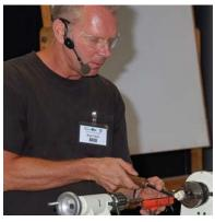
The first thing he demonstrated was drilling a hole in the side of a blank and then turned a piece of holly to back the inlay as the light color works much better than a dark color. He adapter the PSI blank chuck to use as a spindle chuck for the holly which is put inside of a brass tube and the tube is inserted into the hole drilled into the blank.
