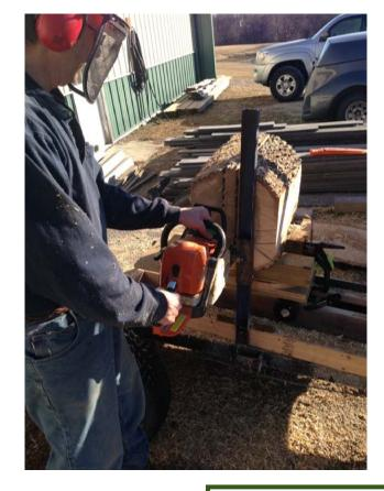
Rick Bywater contributed this to Woodchips. Don Frank cutting ash bowl blanks for the club's silent auction - this contraption allows Don to make straight cuts down on both sides of the pith. The modified bracket is bolted to the chainsaw and slides down as Don makes the cut.
