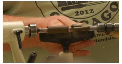
Shaun didn't know that the skew was hard to use so he started using it and it works very well on pens. Lots of turners start with pens. He sharpens it so that the edge of the bevel is rounded off and finds that it is much easier to use that way and makes turning pen blanks much easier and there is no scraping being done, only cutting. OK, the parting tool didn't get shown - it parts things - duh.
