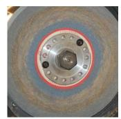
He uses as jig (One Way)to that he gets repeatable results. The one he uses has a tip that swings across the face of the wheel and he can screw the tip a little at a time so that the entire face of the wheel attains a uniform finish and is true. It is also a good ideas to make sure that the wheels are balanced. He uses the One Way system to accomplish this.
