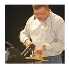
The skew - tends to use a hone but when it gets dropped you have to sue other methods. He uses a belt sharpening system which he made a "quick and dirty" jig for but he gets repeatable results. A word about safety - the particles coming off a stone don't break down so be concerned about your lungs and wear a mask.
