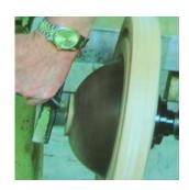
He uses the tail stock to assist in centering. If you are turning a delicate bowl, be cautious about the pressure you apply for holding as the jaws could crack the bowl. The edges of the groove cut into the wood are angled at about 1-2 degrees. After secure, finish the bottom and you are done.
