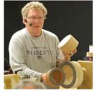
Chucks can be made from PVC and the seal is made from as rubber floor mat. He uses 5 min epoxy to glue.
