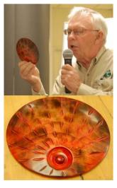
Speaking of off-set turning - **Bill Kuhlman** brought this fine example in. It is a piece of Maple. It started out as 3/4" thick, front turned off-set, reversed and held in place with hot glue complete the back. The finish was done with a torch which burned away the soft wood, lightly sanded, used red anilne dye, used a carving tool to cut in the starburst lines, and then used 2-3 coats of lacquer to complete the piece.
