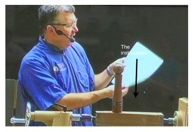
Get the blank to round and then put a tenon on one end. Make sure that you have a good flat edge on the tenon so that the chuck will really be able to hold the wood tightly. After that, start making some measurements so that you will have an ideas of the top and the body and where the mechanism is s to go. When turning - remember speed is your friend, you'll get a better cut.
