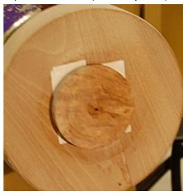
Rick said that all kinds of tools can be used for this turning. Whatever you use best. He used a detail gouge, a round skew, and a negative rake scraper. Has also used his bowl gouge a lot. The back side is turned first. The back side is pretty flat with a gentle curve at the edges.
