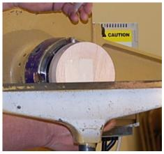
The piece is removed from the pin chuck and remounted on a flat surface in another chuck. Using the double stick tape, it is mounted off center.
