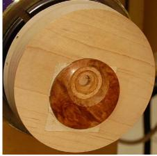
A forstner bit cuts the hole. Then the hole is beveled and finished.
