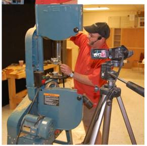
It is very important to make sure that the blade lines up properly because the blade's life with be shorted if not.
