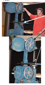
When working on the saw, it is easier to remove the table first. Then give it a good brushing off, inspect the tires. If they are getting loose replace it not very expensive. Some of the typical problems are vibration which can be caused by a bad belt or poor tires on the wheels.
