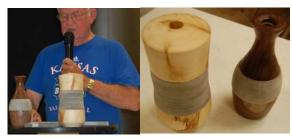
Dale Darnell - brought two forms where paper was used in the center. The wood was aspen and the center was made from layered paper. He did it from an article he read. The first one he did he thought he would break his lathe putting pressure on it and thought he had it tight enough but when it dried, the center was pretty loose. For the second one he ended up with a process using a long threaded rod and a cheater and the second one was much tighter. Much happier with the results.
