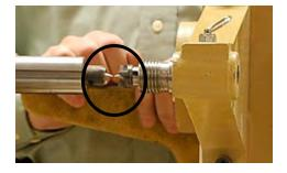
Bring the tail stock up to the head stock (with centers in both) to make sure that this alignment is correct. This is especially important in a new lathe. The parts of the headstock and the tail stock can be cleaned with mineral spirits.
