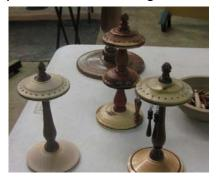
tance between the rim of the carrier and the drilled holes, that it be small enough so that earrings could be put through the holes and hang freely. The spindle was turned as one piece and then parted in two to complete the center post. The pieces are then ready to be finished and assembled. An intresting and informative demonstration Bill.
