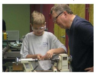
of spindle turning, the boys were on their way. Then they were assigned to a lathe and a KCWT member to help them turn a pen. First they mounted their blanks on the mandrels and started roughing the blanks. Next the shape was worked on and refined. Then the pens were sanded smooth and finished with a wax finish. The blanks were removed from the lathe and another club member helped
