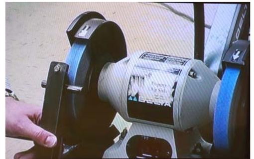
One of the most important things, as a goal, is to have repeatable results and he is showing how to do that tonight. 6-8K surface speed/min on the grinder is important but get rid of the gray wheels as they are too porous. He uses ceramic wheels on his grinder. He also likes his wheels to be clean but the handheld ones are not ones he favors. Friable wheels are best as they wear away and present cleaner material to the tool.
