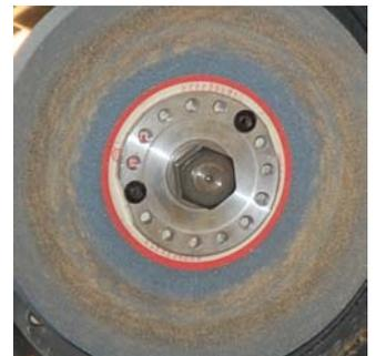
He uses a jig (One Way) so that he gets repeatable results. The one he uses has a tip that swings across the face of the wheel and he can screw the tip a little at a time so that the entire face of the wheel attains a uniform finish and is true. It is also a good idea to make sure that the wheels are balanced. He uses the One Way system to accomplish this.
