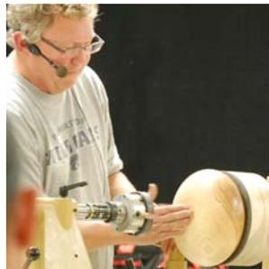
You can make chucks from wood but they need to be sealed and sprayed with urethane. He uses a chuck with an adaptor on the tail stock to center the piece on the vacuum chuck.
