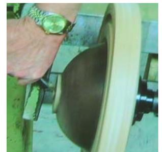
He uses the tail stock to assist in centering. If you are turning a delicate bowl, be cautious about the pressure you apply for holding as the jaws could crack the bowl. The edges of the groove cut into the wood are angled at about 1-2 degrees. After secure, finish the bottom and you are done.
