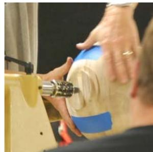
You might need to use some tape of the bowl has some leaks because of inclusions or it's thin. The tape helps set up and sustain the vacuum to that finishing can be done.
